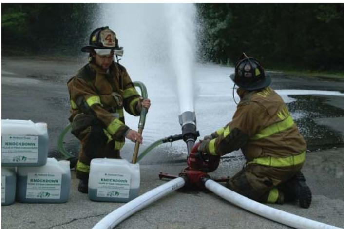
**Figure 5:** Example of a Portable Foam System. Photo Credit: Kidde Fire Fighting - National Foam
