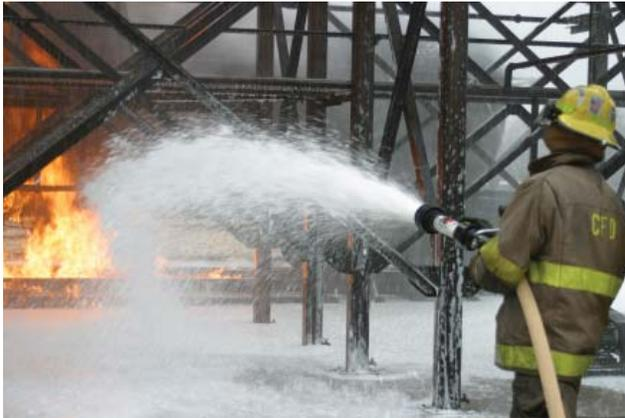
**Figure 6:** *Manual Discharge of Low-Expansion Foam Through a Hose Line. Photo Credit: Kidde Fire Fighting - National Foam*
