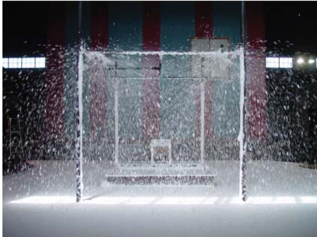
**Figure 14:** *Compressed Air Foam Discharging From Fixed System. Photo Credit: Fireflex Systems Inc.*
