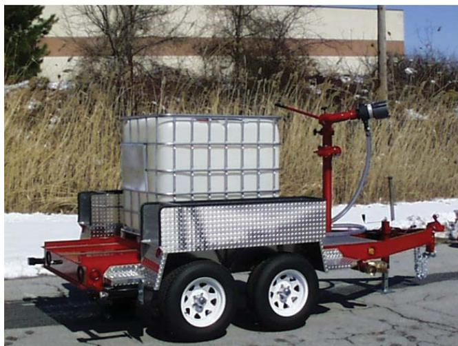
**Figure 3:** *Example of a Mobile Foam System. Photo Credit: Kidde Fire Fighting - National Foam*
