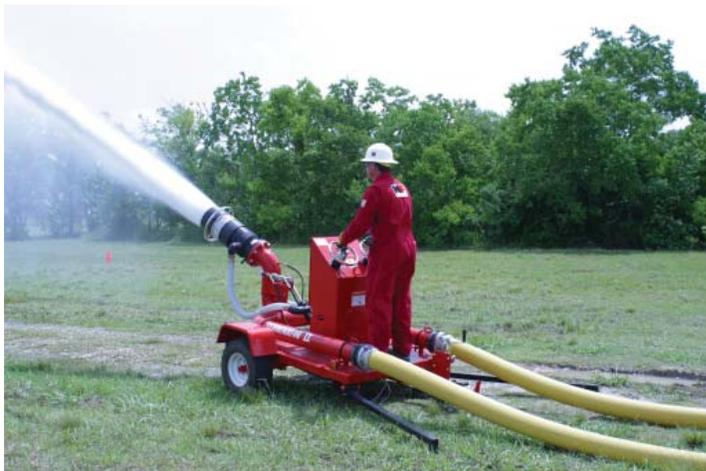
**Figure 4:** Example of a Mobile Foam System. Photo Credit: Kidde Fire Fighting - National Foam
